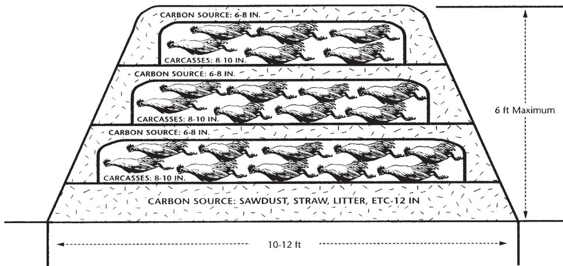
Figure 7. Cross-section of windrow
