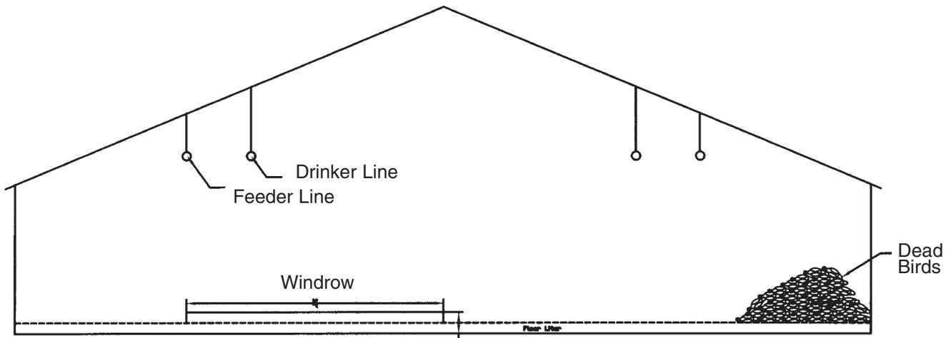
**Figure 3.** Create a windrow 12 feet wide with a base on one side of the house. Make sure outer edge of the windrow does not go beyond feeder line boundary.
